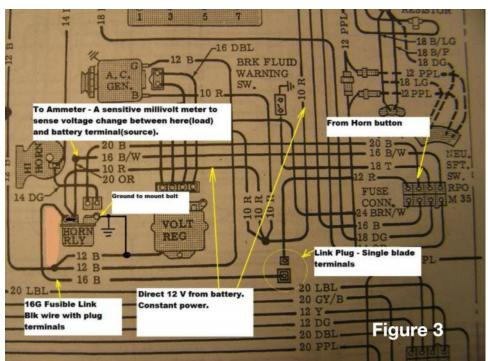
The 1966 CSM (and other years) Wiring Diagram is misleading and shows the Black (Ground) as being attached to the Buss Bar, not the Mount Bolt. This mis-wire would cause a dead short between Power and Ground and may be your fault.
