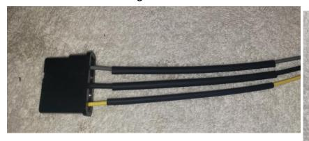
When done, you can test your work with a 12v test light. You should have power on the yellow wire when you turn your key to on or accessory position. The grey wire should be tied to the headlight rheostat and should dim with all the other dash lights when you turn the headlight knob. Check the black wire with a continuity tester to make sure that it goes to ground.
