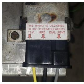
Plug your factory radio back in, and assuming you have your speakers hooked up correctly, you can be listening to your favorite radio station and pass your operations test for radio function!
